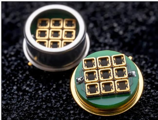
Fig. 1: Infrared emitter matrix with 3x3 individually controllable elements in a standard TO-8 housing for remote sensing applications.
